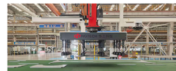
Xinneng Shipbuilding Joint Workshop Intelligent Cutting and Material Handling Production Line
