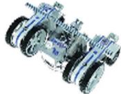
Wall-climbing rust removal robot
